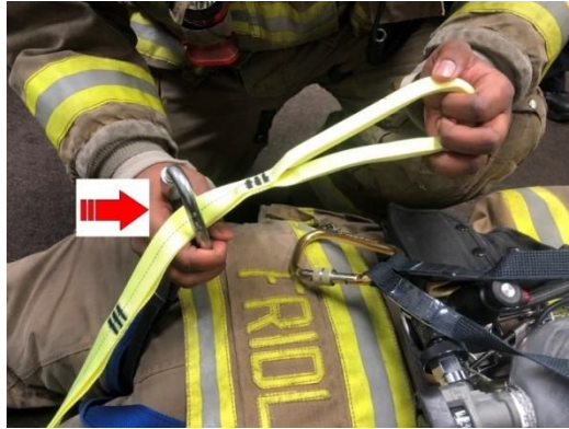
NOTE: Feed rescue strap handle through Tri-Link
